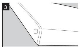
Slide the Larder Fridge door down about 15cm [6"] and off the top hinge pin and lift away from the Freezer.
